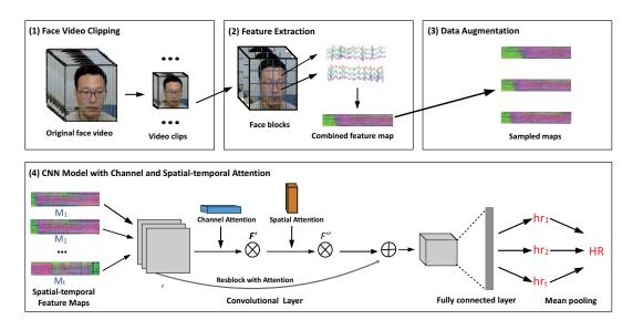
Fig. 3. Overview of the proposed end-to-end trainable approach for rPPG based remote HR measurement via representation learning with spatial-temporal attention.
