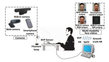
Fig. 3. Devices and setup used in collecting VIPL-HR.
