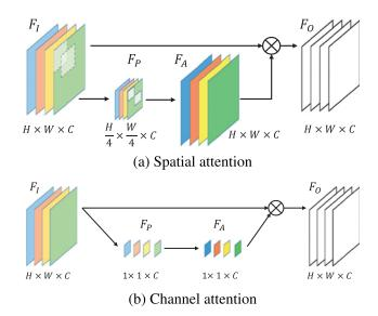
Fig. 3. Attention module for image restoration task: (a) Spatial attention and (b) Channel attention.
