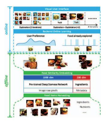
Fig. 5. PlateClick system pipeline [30].
