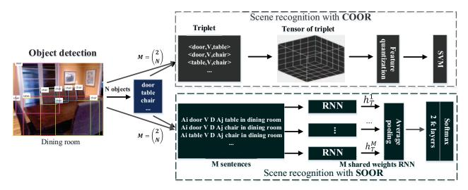
Fig. 2. Framework of scene recognition with COOR and SOOR. N objects are detected to generate  $M = \binom{2}{N}$  triplets and sentences. The triplets are converted into COOR, and then fed to classifiers. All the sentences of (SOOR) are first encoded with RNN, and then pooled to the global vectors, which are finally fed to the scene classifier. Different types of relations, such as V, D, A, are introduced in subsection IV-A.
