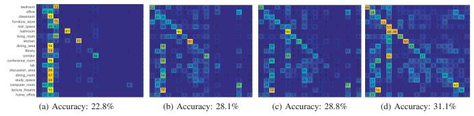
Fig. 5. Confusion matrices, evaluated with annotated objects from ground truth, (a)  $P_S^I$  in Eq. 2, (b)  $P_O^I$  with SVM, (c)  $P_{OO}^I$  with SVM, (d)  $P_{COOR}^I$  with SVM. The horizontal and vertical coordinates are symmetric.
