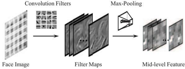
Figure 4: The image feature extraction process.
