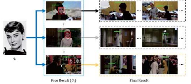
Fig. 10. Framework of the 3rd-place solution in Person Search. Firstly, the preliminary collections of candidates  $G_i$  corresponding to the  $i$ -th query  $q_i$  are gotten. Then similar instances in all candidates are searched according to the ReID features.
