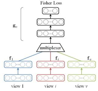
Figure 1. An overview of Multi-view Deep Network (MvD-N). MvDN consists of two sub-networks, the view-specific sub-network  $\mathbf{f}_i|_{i=1}^v$  and the common sub-network  $\mathbf{g}_c$ , along with a discriminant Fisher objective.
