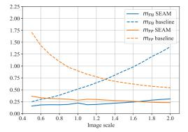
Figure 6. The curves of over-activation and under-activation. Lower  $m_{FN}$  curve represents fewer under-activation regions, and lower  $m_{FP}$  represents fewer over-activated regions.
