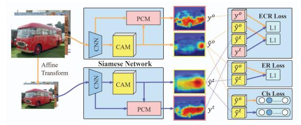
Figure 2. The siamese network architecture of our proposed SEAM method. The SEAM is the integration of equivariant regularization (ER) (Section. 3.2) and pixel correlation module (PCM) (Section. 3.3). With specially designed losses (Section 3.4), the revised CAMs not only keep consistent over affine transformation but also well fit the object contour.
