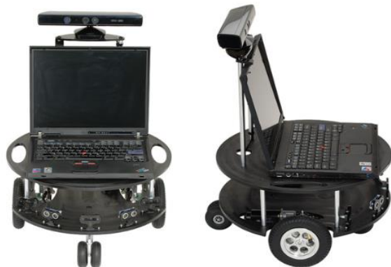
(a) RGB-D data collection robot
