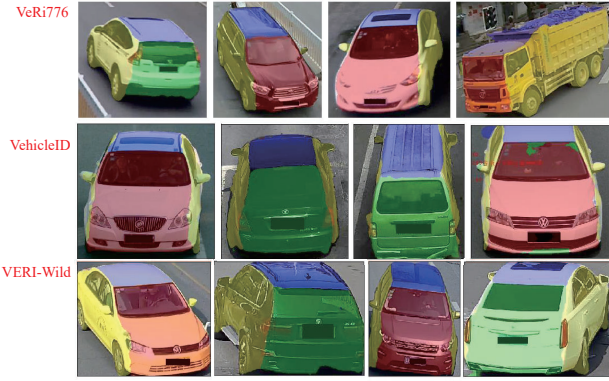
Figure 3. Examples of our parsing result on three main vehicle ReID datasets. The red, green, yellow and blue masks denote the front, back, side and top view of the vehicle respectively.
