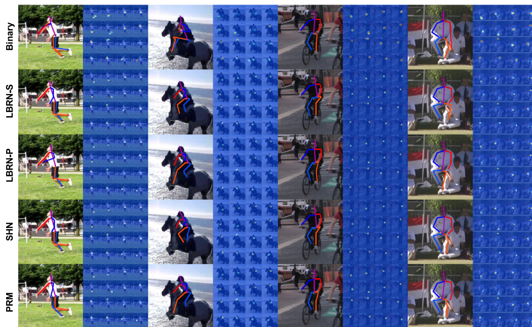
Fig. 5. The example output of pose estimation from different networks. The results of LBRN are similar to that of the full-precision network and outperform that of the full-binarized residual networks. On the left of each image, the final pose estimation is provided after the max activations across each heatmap. On the right we can see all the heatmaps of different joints.
