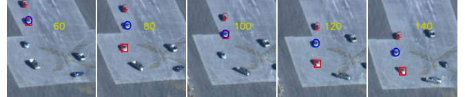
Figure 9: Tracking results on “egtest01”. Red rectangles are for the covariance matrix and blue circles for Sigma Set.
