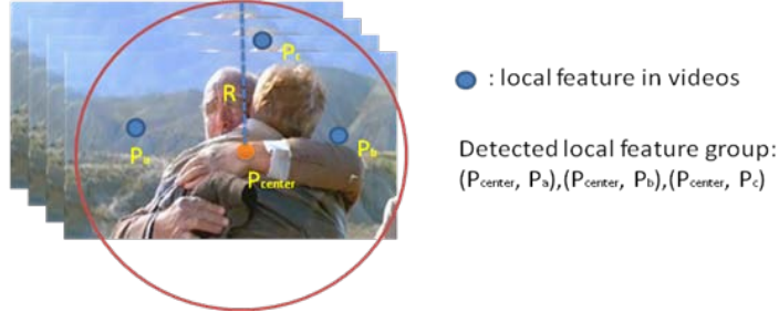
Fig. 3. The feature group detector. It extracts the local features positioned in the radius R and constructs the feature groups.
