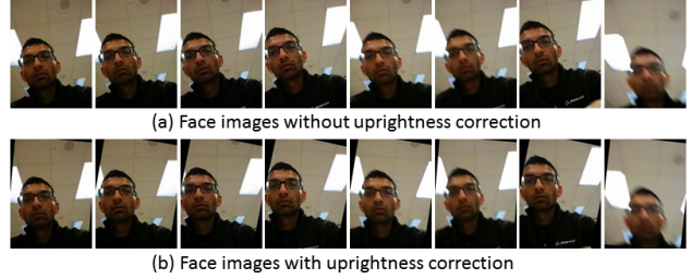
Figure 5. Examples of face image orientation correction using gyroscope, accelerometer and magnetometer data. (a) Captured face images, and (b) corrected face images in which faces are kept upright during the rotation of the mobile device.
