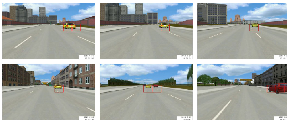
Fig. 6. Vehicle detection examples in the driving simulation system. (For interpretation of the references to color in this figure caption, the reader is referred to the web version of this article.)
