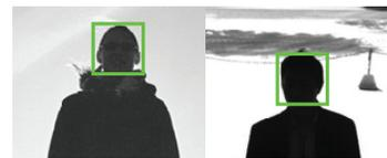
Fig. 1: Due to dramatic lighting variations, face images captured in a CCTV system might be of Low Gray-scale Resolution (LGR).
