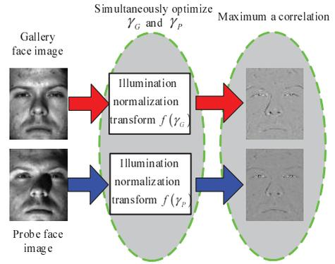
Fig.2 Illustration of optimizing the illumination normalization for a gallery and a probe face images by maximizing a correlation between them.
