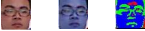
(a) detected face; (b) face in YcrCb color space; (c) pixel clustering results
