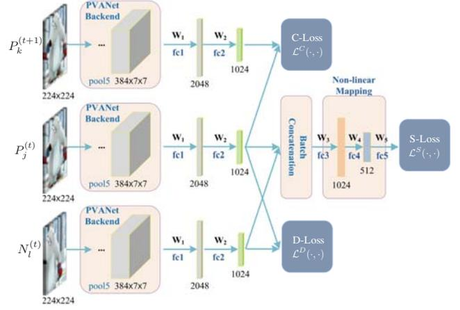
**Fig. 2:** CD CNN Structure for Offline Joint training
