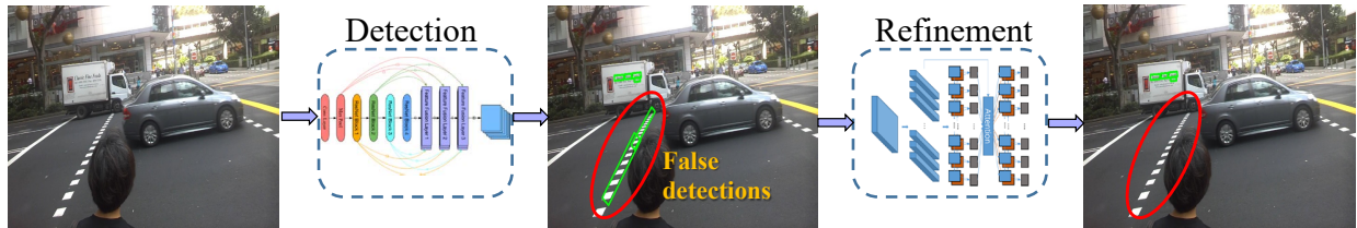
Fig. 2: The pipeline of the proposed scene text detection method, consisting of an initial text detection followed by an attention-based text vs. non-text refinement.
