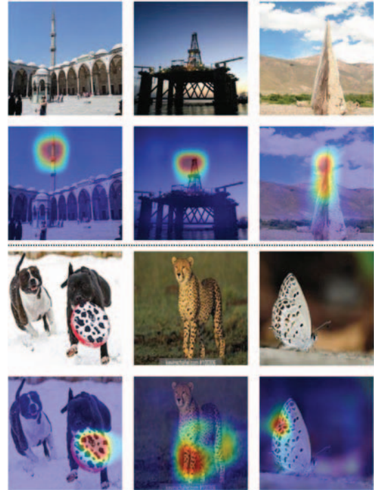
Fig. 10. The heatmaps of activations on two attributes (filters). The top row shows the original images and their activation heatmaps on the attribute “sharp,” and the bottom row corresponds to the attribute “spotty.” In the heatmaps, warm color indicates high activations and cold colors indicate low activations. The attributes here have high activations at the expected parts in the images and low activations elsewhere, even though the highly activated areas correspond to different object categories. This figure is best viewed in color.
