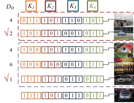
Fig. 2. Hashing system built by using MKLSH. Images in the red dashed box and purple dashed box denote the ImageNet data and Web data, respectively. The bottom image is the query input which can be the labeled training image. D_H is the Hamming distance of the binary codes. The images marked by “red√” is the returned images.
