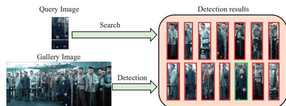
Figure 1. The consistency problem in the detection stage. The red boxes indicates non-query pedestrians and the green box indicates the query target in gallery image. The person detector produces bounding boxes of each pedestrian, which leads to a large gallery size for the re-ID stage.
