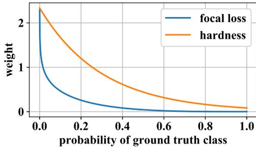
Figure 5. The weight varied with the probability of ground truth class for our hardness factor and the focal loss.
