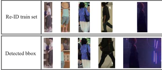
Figure 2. The consistency problem in the re-ID stage. The first line are examples from re-ID train set, the second line are corresponding detection results. In actual search process, the detected bounding boxes are more vulnerable to problems of misalignment, occlusions and body part missing.
