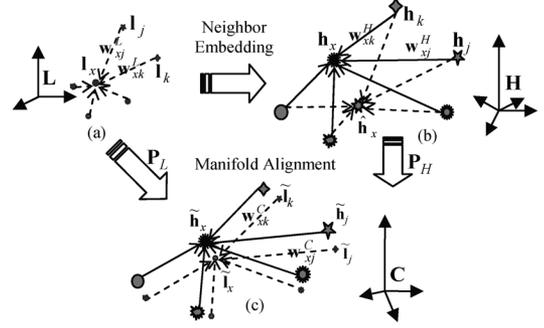
Fig. 2. Neighbor embedding based on manifold assumption and manifold alignment.  $\tilde{\mathbf{x}}$  is the projection of  $\mathbf{x}$  on CM.
